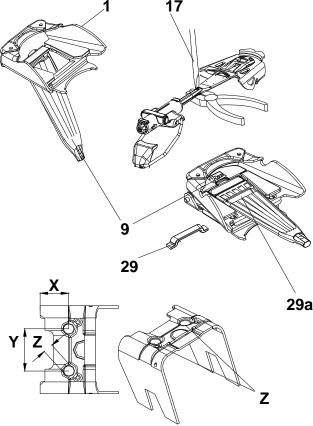
Important: If the adjustment of the binding spring pressure is preset to a value which exceeds the recommended value, a pretemporary failure of wear parts, such as the tension strap, is very likely!
